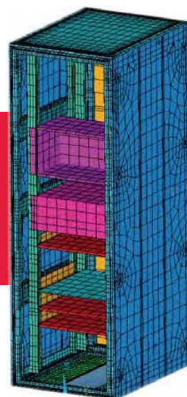
F.E. model - mesh and stress analysis
