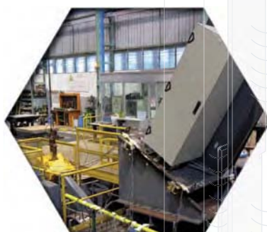
Cabinet tested to MIL-STD-901D
