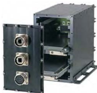
7 slot 3U VPX Titan chassis, available with Birtcher® 3U VPX clamshell, vertical and horizontal mounting options; various modular design options available
