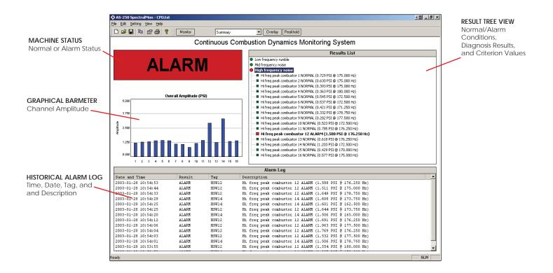
In many industrial applications, there is a need to monitor the dynamic characteristics of large machinery (such as turbines and compressors) or processes (such as steel and paper production).
