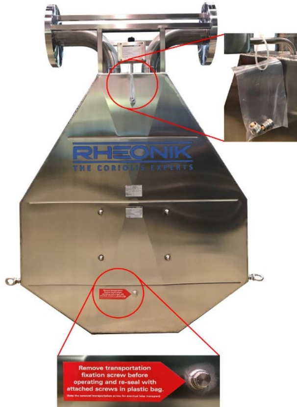
Figure 6: Transportation fixation screw and plugs
