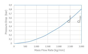
0 – 3000 kg/min water, sensor with P1 pressure rating. Higher viscosities create higher pressure drop
